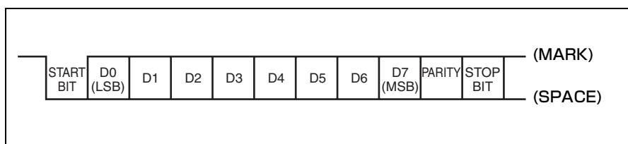
1 START BIT + 8 DATA BITS + 1 PARITY BIT + 1 STOP BIT
