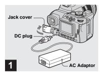
Open the jack cover, then connect the AC Adaptor (supplied) to the DC IN jack of the camera.
