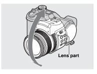
You can adjust the angle by turning the lens part upward up to 70 degrees and downward up to 30 degrees.
