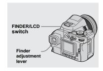
With the FINDER/LCD switch, you can choose to shoot either using the finder or the LCD screen. When you use the finder, the image does not appear on the LCD screen. Adjust the finder adjustment lever until the image appears clearly within the finder, then shoot the image.
