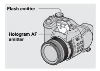
The flash automatically pops up and strobes when the surroundings are dark. Close the flash by hand after using it.
