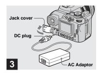
Open the jack cover and connect the AC Adaptor (supplied) to the DC IN jack of your camera.
