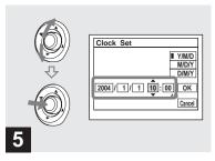
Set the desired numerical value by moving the multiselector to ▲/▼, then press the center.
