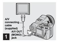
→ Connect the supplied A/V connecting cable to the A/V OUT (MONO) jack of the camera and the audio/video input jacks of the TV.
