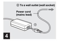
Connect the power cord (mains lead) to the AC Adaptor and then to a wall outlet (wall socket).
