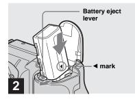
→ Install the battery pack, then close the battery/"Memory Stick" cover.
