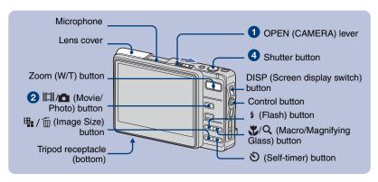
Open the lens cover by sliding the OPEN (CAMERA) lever.
