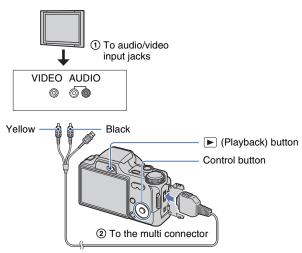
If your TV has stereo input jacks, connect the audio plug (black) of the cable for multi-use terminal to the left audio jack.
