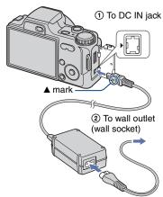
You cannot charge the battery pack by connecting the camera to the AC-LS5K AC Adaptor. Use the battery charger (supplied) to charge the battery pack.
