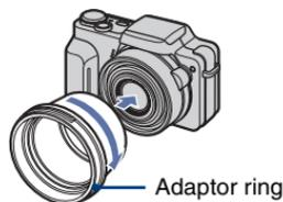
2 Position the lens hood as shown below and turn the lens hood clockwise until it clicks.
