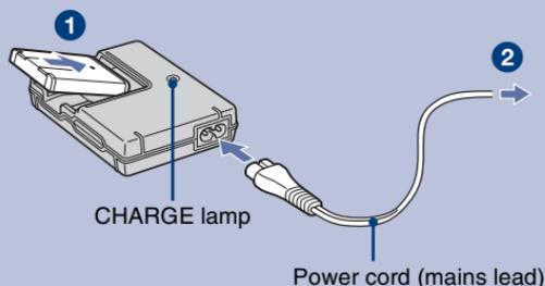
**1** Insert the battery pack into the battery charger.
