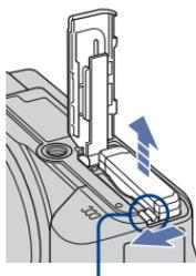
Slide **the battery eject lever**. Be sure not to drop the battery pack.
