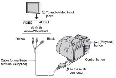
If your TV has stereo input jacks, connect the audio plug (black) of the cable for multi-use terminal to the left audio jack.
