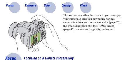
When you press the shutter button halfway down, the camera adjusts the focus automatically (Auto Focus). Remember to press the shutter button only halfway down.
