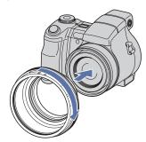
② Turn the position ring and position the indicator of the adaptor ring to the indicator of this camera, as illustrated below.
