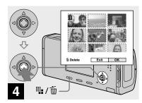
Press : / ( Delete) and select [OK] with ▶ on the control button, then press ●.
