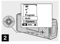
⇒ Select (Camera) with on the control button, then select the desired mode with \( \Lambda \rightarrow \).
