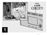
→ Set the mode switch to ►, and turn on the power.
