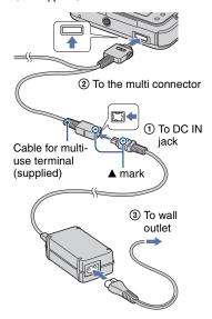
You cannot charge the battery pack by connecting your camera to the AC-LS5K AC Adaptor. Use the battery charger to charge the battery pack.
