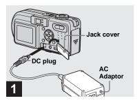
→ Open the jack cover and connect the AC-LS5 AC Adaptor (supplied) to the DC IN jack of your camera.
