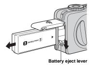
Open the battery/"Memory Stick" cover. Slide the battery eject lever in the direction of the arrow, and remove the battery pack.
