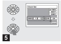
→ Set the numeric value with A/▼ on the control button, then press ● to enter it.
