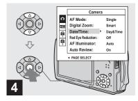
→ Select the date and time setting with A/▼ on the control button, then press ●.
