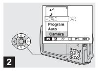
⇒ Select (Camera) with < on the control button, then select the desired mode with △/▼.</p>
