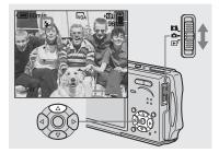
→ Set the mode switch to n, and press (4) on the control button repeatedly to select a flash mode.
