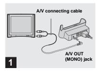
Connect the A/V connecting cable (supplied) to the A/V OUT (MONO) jack of the USB cradle (supplied) and the audio/video input jacks of the TV.
