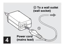
Connect the power cord (mains lead) to the AC Adaptor and to a wall outlet (wall socket).
