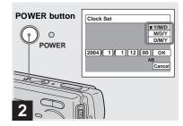
Press the POWER button to turn on the camera.
