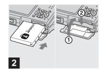
→ Install the battery pack, then close the battery/"Memory Stick Duo" cover.
