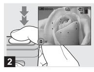
Center the subject in the frame. Press and hold the shutter button halfway down, then press the shutter button fully down.
