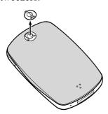
2 Slide the back over of the player down, and then lift up, as shown by the arrow below.
