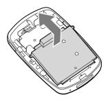
5 Remove the two screws at the edge of the battery chassis.
